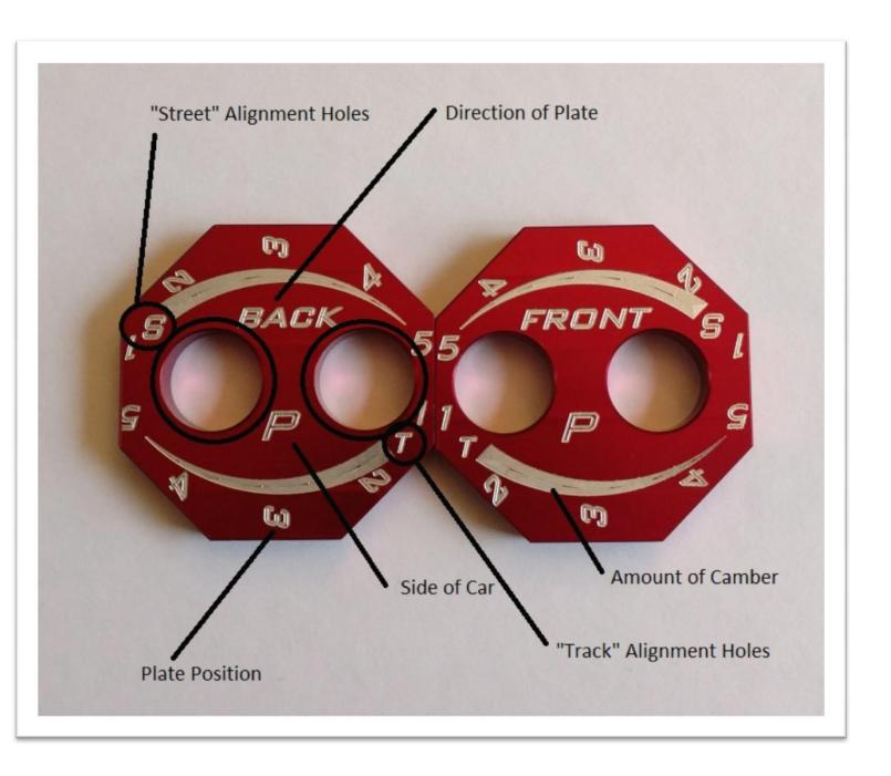
**Side Of Car** – Each pair of plates is marked with either a "P" or a "D". All plates with a "P" on them will be installed on the Passenger side of the car and plates with "D" on them will be installed on the Driver side of the car.
